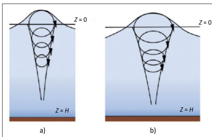
**Figure 2.** Structure of surface waves
