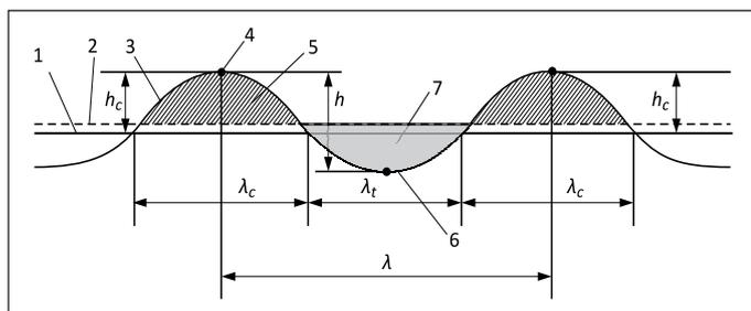
**Figure 1.** Wave profile and its elements: 1 – static level, 2 – average wave line, 3 – wave profile, 4 – wave top, 5 – wave crest,  $\lambda_c$  – crest length,  $\lambda_t$  – trough length,  $h$  – wave height,  $h_c$  – crest height
