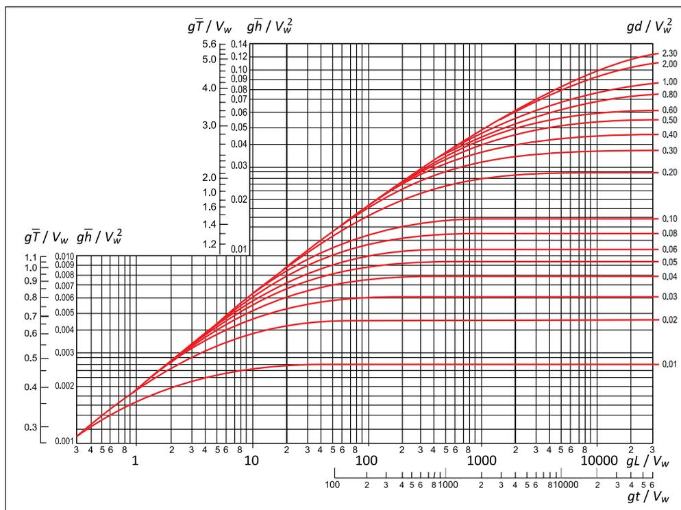
Figure 3. Graph for determining the elements of wind waves
