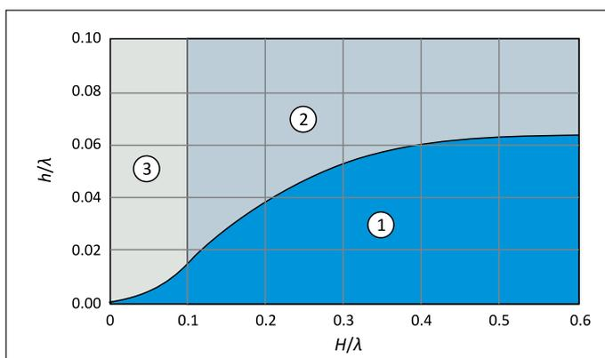
**Figure 4.** Diagram of applicability of: Airy wave theory (1), Stokes wave theory (2) and cnoidal waves (3)
