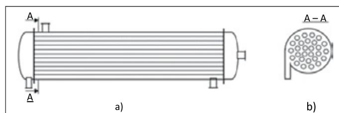
**Figure 2.** Shell-and-tube heat exchanger working under the influence of centrifugal force
