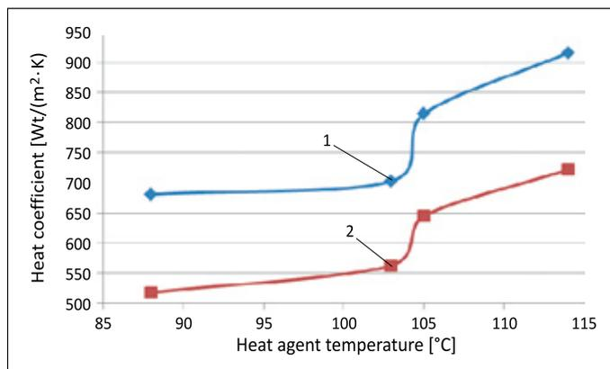
**Figure 7.** The effect of the change in the temperature of the heating agent on the individual heat transfer coefficient  $\alpha_2$  and overall heat transfer coefficient  $K$ : 1 – individual heat transfer coefficient,  $\alpha_2$ ; 2 – overall heat transfer coefficient,  $K$
