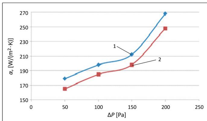
**Figure 4.** Effect of pressure change on the individual heat transfer coefficient  $\alpha_2$  and overall heat transfer coefficient  $K$ : 1 – individual heat transfer coefficient,  $\alpha_2$ ; 2 – overall heat transfer coefficient,  $K$
