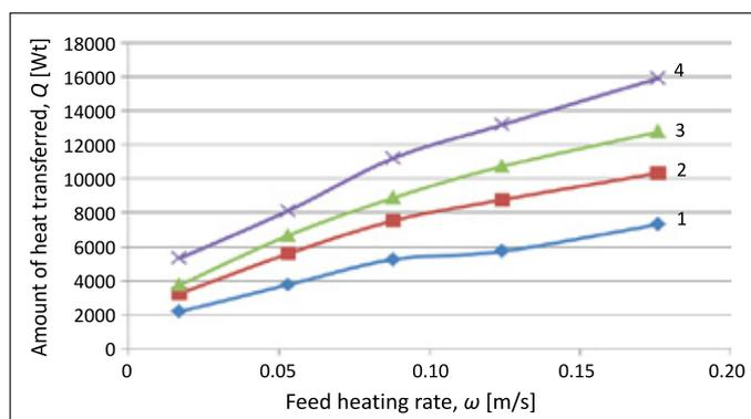
**Figure 3.** The effects of temperature, pressure of the heat agent, and changes in the rate at which raw materials are heated on the amount of heat:
