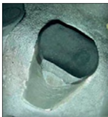
Figure 5. Structure of fixed cutters, zone of wear degree and its concentration on the fixed cutter (Neskoromnykh et al., 2020)
