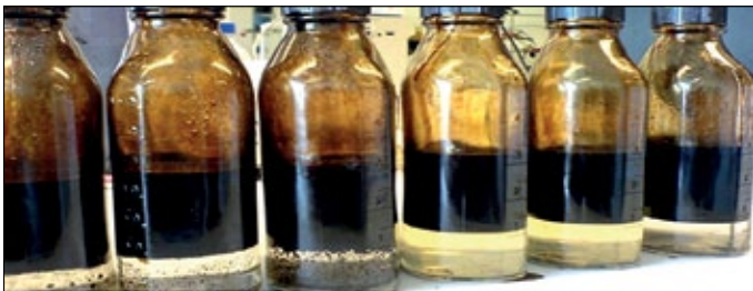
Figure 10. Visual results of crude oil demulsification after treatment with the KA-3 and KA-2 compositions at the optimal concentration
