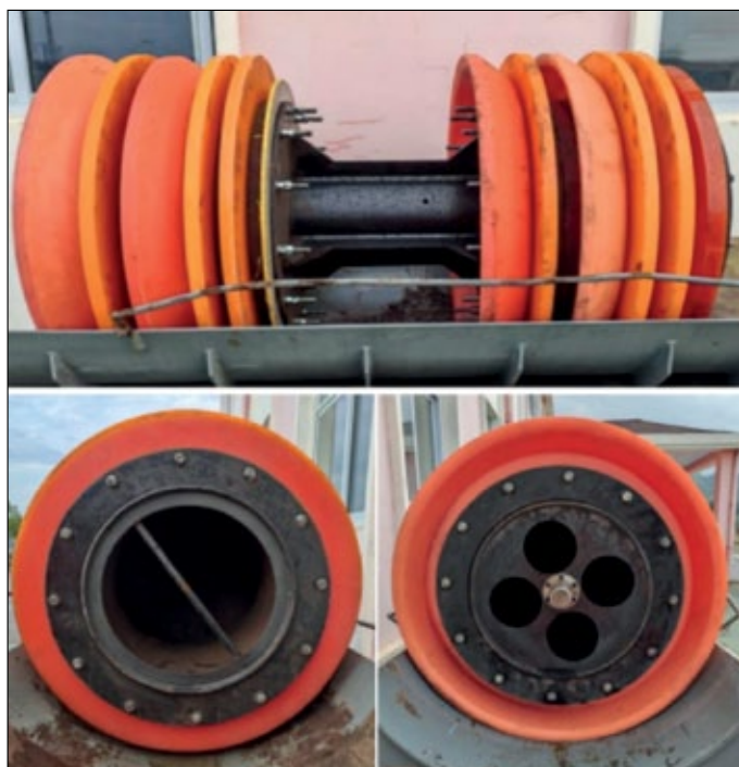
Figure 3. Appearance of the pipeline inspection gauge
